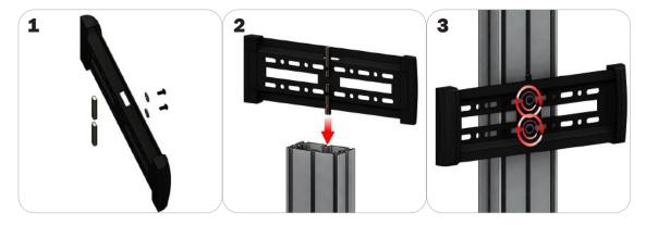
Locate all components needed to assemble the monitor mount with the channel connection B method. You will need (1) monitor bracket, (2) LN-LCD-SCW, (2) LN-100, and (2) washers.
