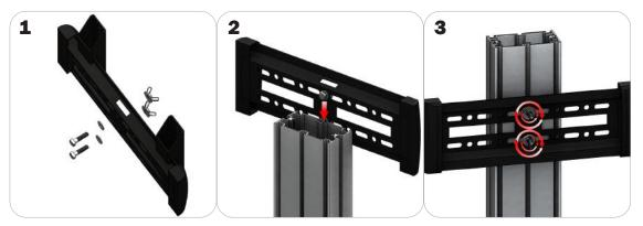
Locate all components needed to assemble the monitor mount with the channel connection A method. You will need (1) monitor bracket, (2) square head bolts, (2) washers, and (2) wing nuts.
