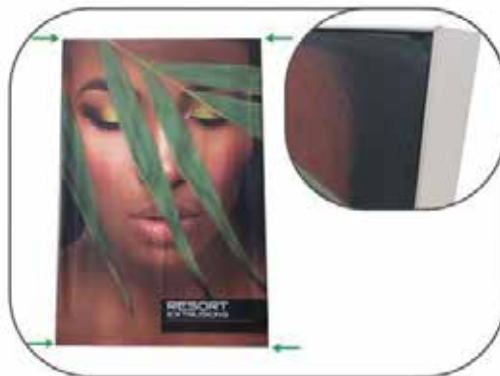
Begin inserting SEG beading at each corner.
