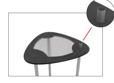
**Step 7:** Secure the first two sections of poles into the top. Slide first shelf onto poles until they rest on push button. Insert the next section of poles and repeat process.
