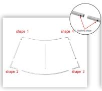
Connect corner sections to straight sections with matching shape codes.
