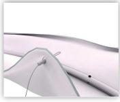
6. Thread cable support through eyelet.
