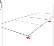
4. Connect feet by pressing and pushing.
