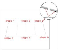
2. Connect corner sections to straight sections with matching shape codes.
