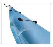
7. Position lights as desired and clamp in place.
