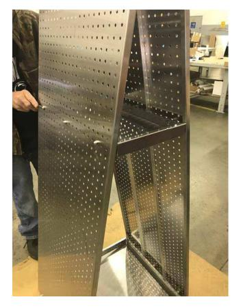
8. Secure the center shelf to the pegboard using acorn nuts.
