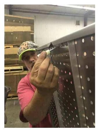
5. Using the Gludots, attach two of the 3/4" spacers together. Place one 2" screw through the center hole at the top of one pegboard panel. Repeat this step and add spacers to first and last peg hole on the top row.
