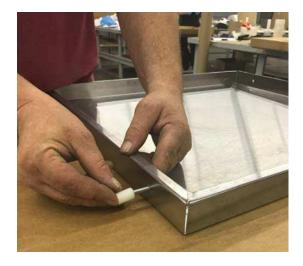
2. Place 1" screws through the pre-punched holes located on the center and bottom shelves. Attach the spacers with GlueDots to the outside of the shelves.
