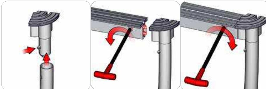
First, press and hold the snap button while you slide it into the tube. The snap button connection is secure when it protrudes through the tube hole. Second, using the allen key tool, disengage the cam lock in the extrusion end and place its teeth into the CB10-R channel. Third, with the cam lock teeth in the channel, use the allen key tool to engage the cam lock. Make a half turn to lock, do not over tighten. Repeat for opposite end.
