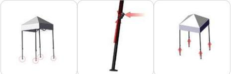
The frame will have four slide locks, one for each corner. When the tent scissor frame is fully extended; make sure the prong of the slide lock snaps into the tube locator hole. Press the lever on the slide lock to disengage the prong from the tube allowing to slide the lock up or down during assembly.
