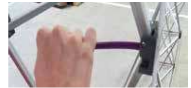
F2. Remove the female arm as in M2.; wiggle side to side and pull out to one side .
