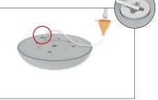
Step 4: Insert the center support pole into base of bubble. Screw the base plate through the bottom of the base into the pole.
