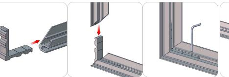
First, insert the corner connector into the extrusion. Then, slide the next extrusion onto the same corner connector. Finally, hold the corner components together and use the provided Allen Key to lock the corner connector in place.
