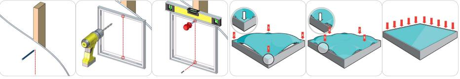
First, find the wall studs and mark it with a pencil. You can use a stud finder to help locate the studs. Second, drill holes on the frame for screw clearance. Do not make the holes larger than the screw heads. Make sure to drill on center for top and bottom horizontal frame runs. Third, level and hold the frame in place lining up the frame holes with the pencil line. Finally, use a hand screw driver to secure the frame onto the wall with screws. (tools and hanging hardware not included)
