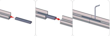
First, insert the straight connector into the extrusion. Then, slide the next extrusion onto the same straight connector. Finally, hold the components together and use the provided Allen key to lock the corner in place.
