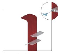
The shelves come semi assembled, just make sure that they are level before you tighten the clamp.
