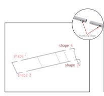
2. Connect corner sections to straight sections with matching shape codes.
