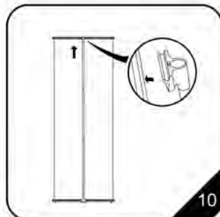
10. The hook at the top of the pole slips into the rear slot of the banner beam. A marker on the beam indicates the beam's centre where the pole should be inserted.
