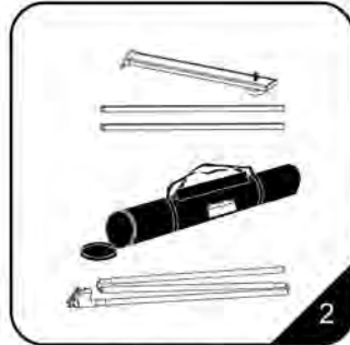
2. The case should contain two pieces base-unit, four pieces of snap-rails and two 3-piece-pole.
