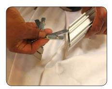
**Step 7** Grab 2 Screw Curved corner Bracket and one Flat Corner Bracket, un-tightening the screws a little bit so the flat corner bracket and the screw corner bracket are flat enough to insert into the angled corners of the frame bars.
