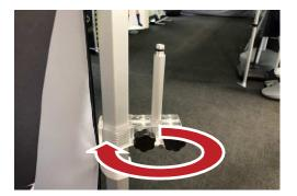
Unscrew the pole pin wing nut, slide the pin through the accessory piece hole, and lock in place with the wing nut.
