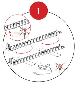
Fit the Bottom Extrusions together.
