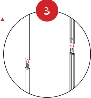
Fit the Top Extrusions together.
