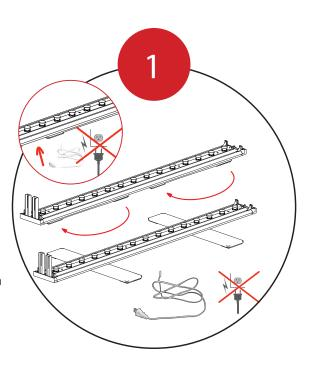
Fit the Bottom Extrusions together.
