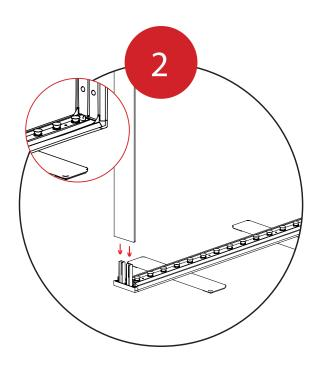
Fit the Side Extrusion Tops Anonto the Side Extrusion
