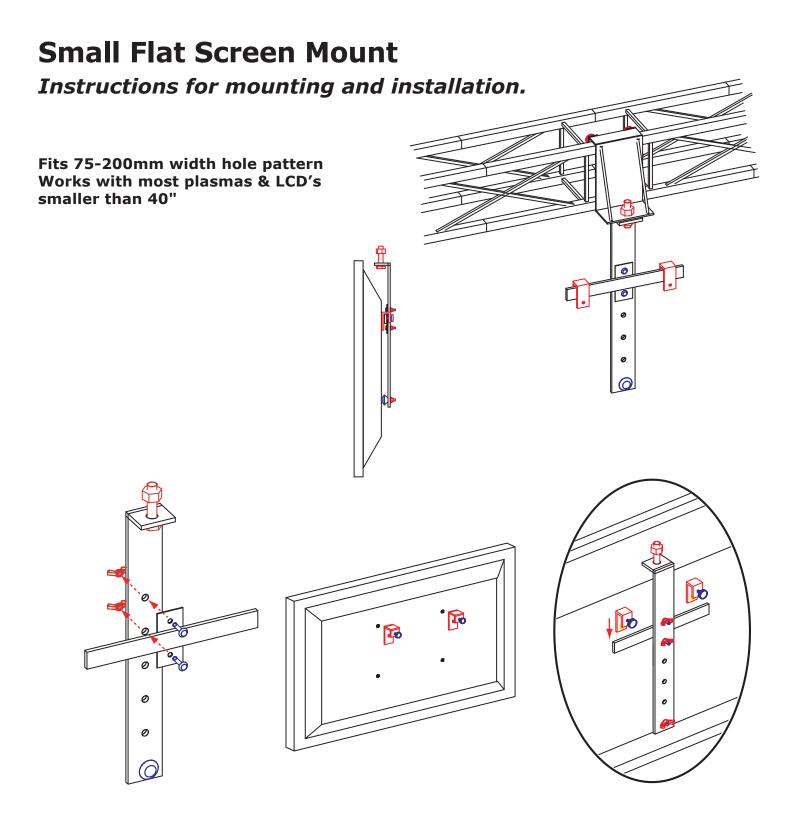
Mount bracket to truss, using the horizontal or vertical bracket provided for your application. Swivel the frame so it's facing the direction desired for your screen, and tighten top bolt to secure. Attach crossbar and plastic spacer at choice of holes on frame, and tighten securely with wingnuts.
