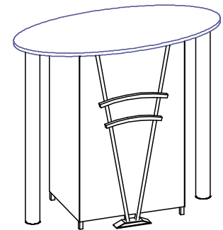
Carefully flip the counter top over and place over the main unit making sure to line up the velcro strips on the underside on the counter top
