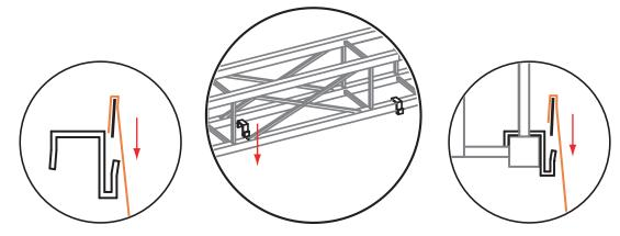
Slide the rigid edge of the banner down into the hook end of the clip, about every two feet, then attach clips onto truss tube.
