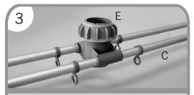
3. Remove 3 Banner Arm Clips from the Lower Banner Arms (B). Fit Lower Banner Arms (C) into the pole's Lower Connecting Piece (E) and put the removed Banner Arm Clips back on. At the Connecting Piece (E), fix the Lower Banner Arms (C) in a central position.
