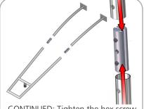
CONTINUED: Tighten the hex screw so the joiner seperates and tightens against the inside of the tubing, locking the joiner & tubing together.
