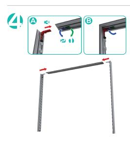
Slide side extrusions into top extrusion channel. Use latch to press down on the L connector. Then press down the second latch to secure.
