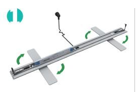
• See numbers on each extrusion piece. Match number together (e.g. 3-3). From the bottom extrusion, twist the feet.
