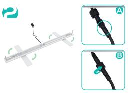
Connect the transformer power cords together. Then tighten the knob to secure the cords.
