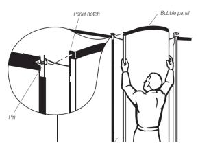
Connect Bubble Panel by hooking the panel notches over the pins at the top of the channels. Align to magnets on channels.
