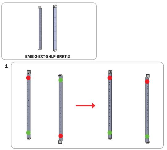
Locate the stickers on the accessory brackets and turn them so they are rotated to the correct direction.
