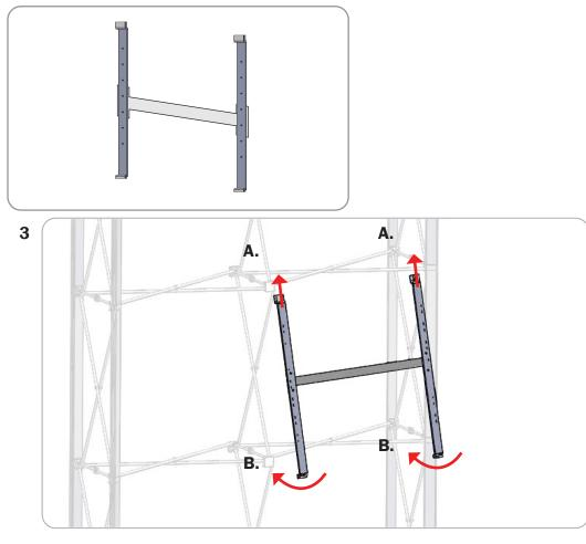
A. Attach the bracket assembly to the Embrace frame by first tilting it up and attaching the top of the scissor brackets to the upper embrace arms. Make sure brackets are the correct orientation before attaching. Follow the strickers on the brackets.
