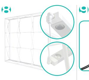
• Plug the Jumper Cords into the top and bottom Edge Lights together.
