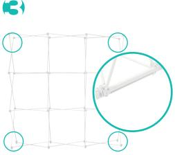
• Connect the top and bottom End Caps on each side of the frame.
