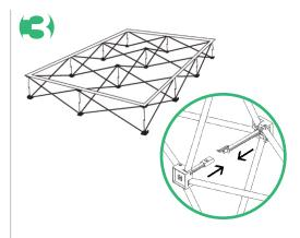
• Make sure hook strips are facing up. Push together all locks on frame to connect.
