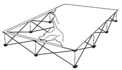
Attach the rest of the graphic by working your way around the frame. Make sure graphic is pulled taut while attaching the hook and loop.
