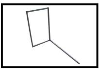
Attach horizontal poles to end frames (Lengths vary between 2', 4' and 6' depending on model)
