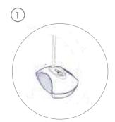
Insert pole into the hole of base as shown in picture.
