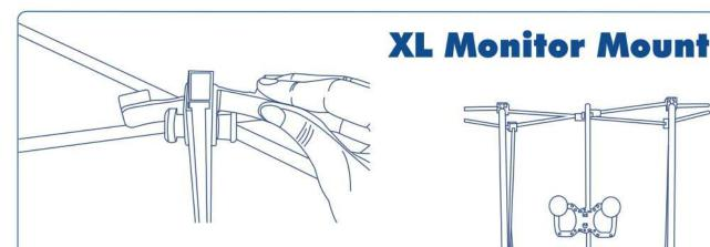
Lift the XL mount above the cross-bars of your desired location, and hang on top and bottom cross-bars at the same time.
