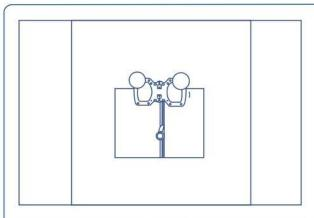
Install fabric/graphic panels on the channel bars. Make sure to have the XL mount go through the opening on the panel.
