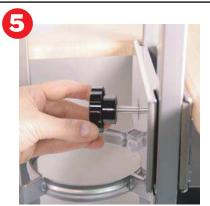
Finish by screwing the black knob/ bolt back into place and tightening.
