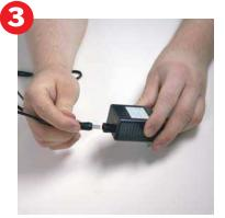
Transformer should already be attached, if not simply plug cord into transformer (make sure transformer is not plugged in).
