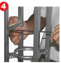
Finish tightening screw with t-tool and repeat steps 2 & 3 for other side of the shelf.
