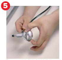
To remove light bulb, hold bulb from sides with fingertips and pull out. (WARNING: allow light to cool off before attempting to change bulb or pack away).
