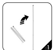
.Unfold the pole and slip the pieces together to assemble it to a rigid pole (the hooked end corresponds to the top and the round end belongs to the bottom base).
