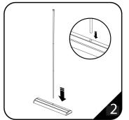
2. The bottom of the assembled pole slides into the round socket in the centre of the base unit.
