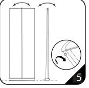
5 .The unit can be levelled by adjusting the threaded feet at the bottom of the base unit.
