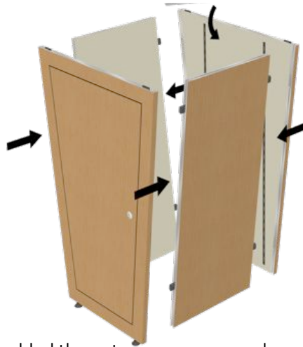
Assembled the octanorm as seen above. Each panel has button that allows to be assembled.
