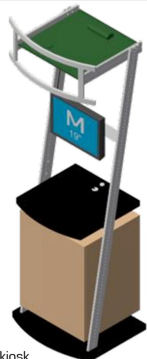
Slide the ceiling in between the octanorm using the groove of the octanorm as a guide.
