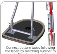
the labels by matching number to number. Slide joiner into tubing so hex screw sits in hole on tubinger.
