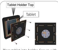
Place tablet into holder. Secure with thumbscrews. Plate on base must be vertical (as shown) to lock properly.
