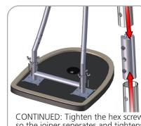
CONTINUED: Tighten the hex screw so the joiner seperates and tightens against the inside of the tubing, locking the joiner & tubing together.
