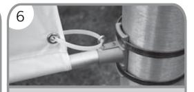
6. Secure the banner by attaching a Zip tie (A) through the Eyelet screw (E) and grommet located on the banner at the top and bottom Aluminum tubes (D).
