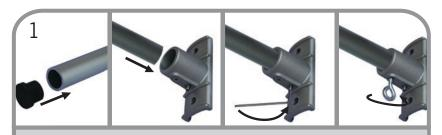
1. Put end cap (F) in Aluminum tube (D) and insert opposite end into the Mounting bracket (C). Use the Allen wrench (B) to tighten the Hex screw (already in place in the mounting bracket). Twist the Eyelet screw (E) to secure tube into place.
