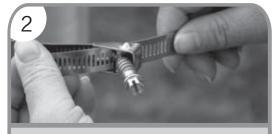
2. Determine the height the top Mounting bracket (C) will be attached and wrap the stainless Steel band (G) around the pole. Bring the end of the Steel band (G) under the screw locking-mechanism. The screw must be in the up position.
