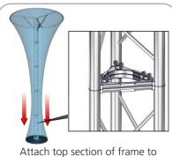
Attach top section of frame to bottom section with base plate and secure using bolts and wing nuts.
