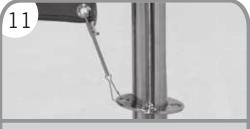
11. Pull the Bungee Cord (I) and attach the Spring Snap (K) to the Connector Plate (F) located at the bottom of the Post (D). Adjust the Tensioner (J) until the Print (L) is taut.
