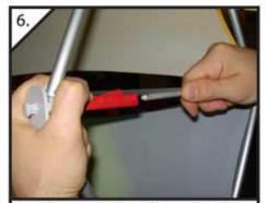
Make sure to manually release all connectors before breaking down.
