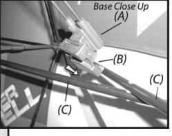
Tip Light (A) back as shown. Fit Base (B) between front and back Scissor Bars (C). Rest the Back of Base (B) under back Scissor Bar (C). Tip Light (A) downward resting the front of base on front Scissor Bar (C).
