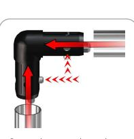
Connect bottom and top tubes to side tubes following the labels.
