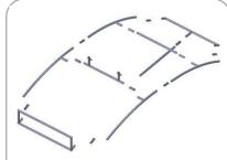
Connect bottom and top tubes following the labels, then connect side tubes. Note tubes with hook & loop on face.
