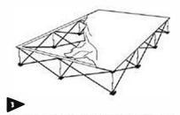
Working in a continuous direction around the frame, attach the rest of the graphic. Make sure the graphic is pulled tout while attaching the Hoolc & Loop.
