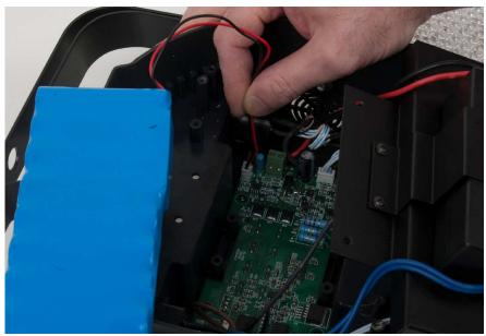
Set the battery and battery cradle to the side. Follow the battery wire to its connection point on the PC board. Disconnect the wire from the PC board and remove the battery.
