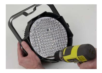
Once the lens cover has been removed, unscrew the 4 phillips screws that hold the LED panel in place.
