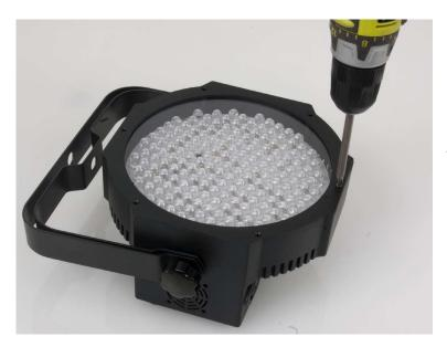
Start by unscrewing the six phillips screws that secures the cover lens.
