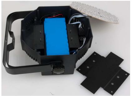
Remove the battery cover to access the battery.
