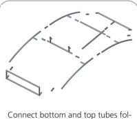
Connect bottom and top tubes following the labels, then connect side tubes. Note tubes with velcro on face,
