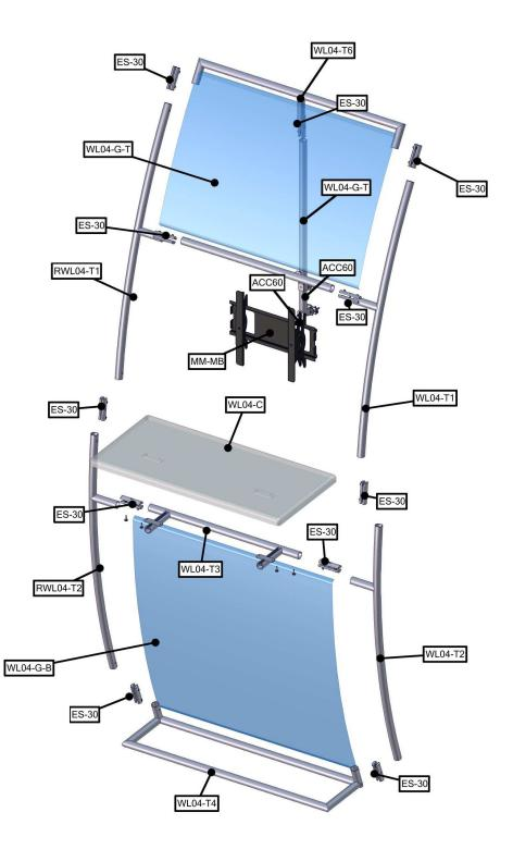
WL04 Frame Assembly: Assemble unit by laying tubes flat on the floor. Connect the tube rails following the labels by matching number to number. See detailed drawing.
