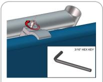
Using provided 3/16" hex key, rotate bolt clockwise to secure accent to top of fabric backwall.
