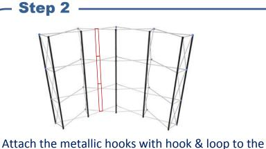
back of the light fixtures and hang on the frame.
