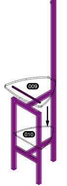
Place and connect counter to the front posts with extrusion locks. Tighten with wrench.
