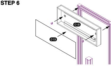
Connect lightbox (with lights pre-assembled inside) to the upper posts with supplied hammer-head bolts. Tighten with pliers or wrench (DO NOT OVERTIGHTEN).
