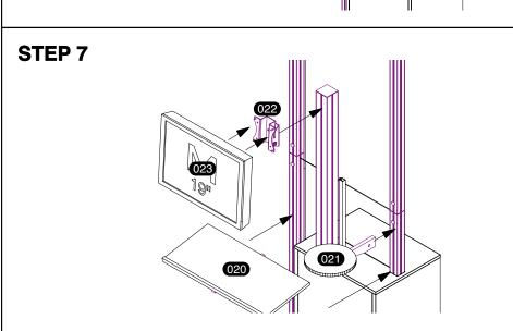
Connect monitor to center post as shown. Attach keyboard shelf and mouse shelf to smaller posts. Engage locks with supplied tool, tightening 1/4 turn to the right.
